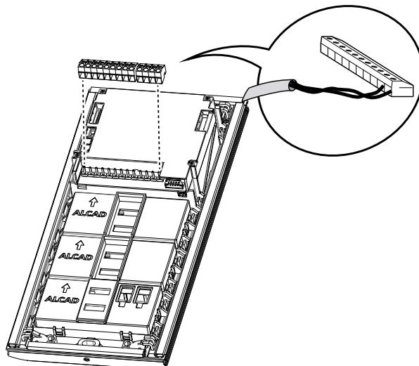
4. When the electrical connections have been made, configure the entrance panels. See SW1 rear switch configuration, page 64.
