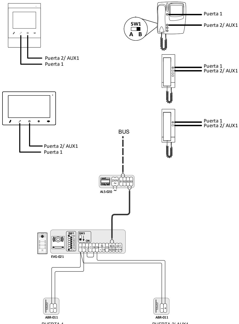
**ACTIVACIÓN LUZ DE ESCALERA MEDIANTE PULSADOR AUX1 DEL TELÉFONO/MONITOR**
