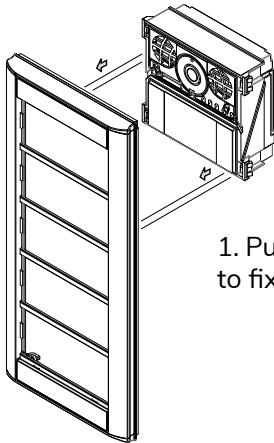
1. Put the main module in position and press firmly to fix it to the frame.
