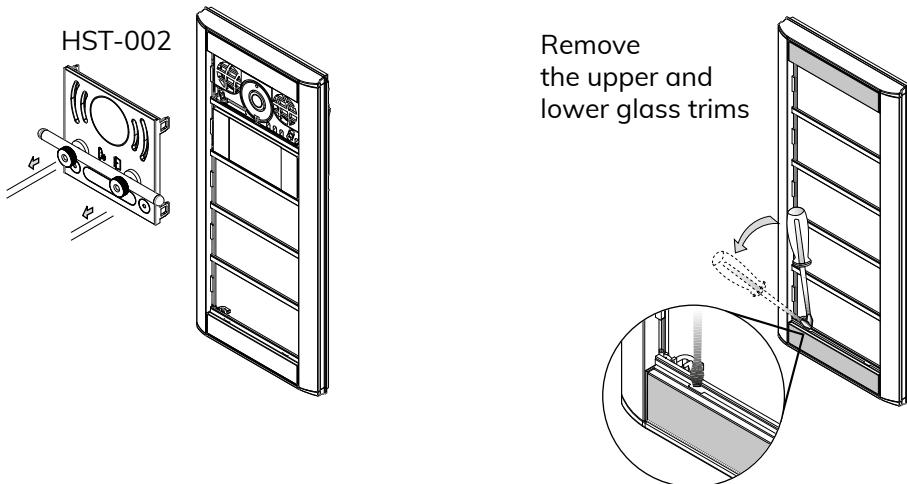
2. Fix the panel onto the hinges of the flush-mounted box.
