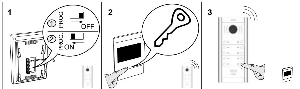
**Note:** Once the monitor is programmed, make sure that the PROG switch is in the ON position.
