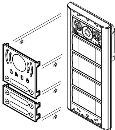
8. How to remove the front glasses with HST-002 tool.
