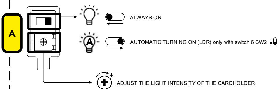
**OPTION 2 - FEEDING THROUGH  $V_{IN}$  - LIGHTING ALWAYS ON**
