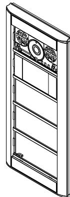
**NOTE:** Use both hands to remove the front glass: hold the removing tool with thumb and index finger and pull gently while resting your hands on the wall for better control of movement. Regarding the 2 windows front glasses: fix the tool on the lower part of the glass.
