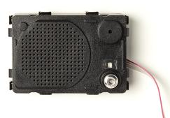
Module with loudspeaker and microphone for entrance panel. It has an 8 ohm speaker with plastic membrane to prevent deterioration over time in outdoor conditions. Also, the robustness of the electret-type microphone against humidity and heat make this module a virtually indestructible assembly.
