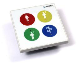
Wall push-button base, touch version, with antibacterial coating, call button, blue code button, auxiliary button and presence button together with green and red, yellow and blue LEDs. This button allows you to make a call and indicate the start and / or end of the presence in the room by pressing the button, while the green LED allows you to identify the room. Wall or surface mount.
