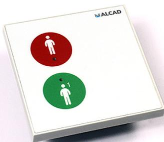
Room touch version peripheral with two buttons: a nurse call button with a red LED and a nurse presence button with a green LED. This peripheral allows patients to call the nurse with the red button. Once initiated the call, the red LED helps to locate the origin of the call easily. The green button is used to either indicate that the nurse is present or to cancel the call. Wall or surface mount.
