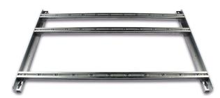
Support frame for 912-series headends with redundant power supplies. It can hold up to 2 power supplies, one amplifier and 7 modules, or 2 power supplies and 8 modules. There is a 47 mm distance between modules to allow for better heat disipation.
